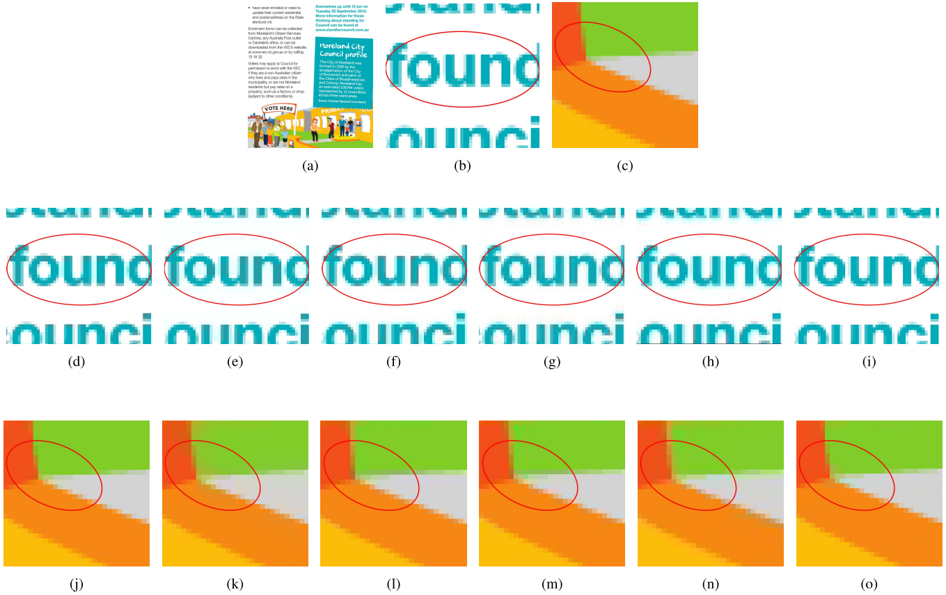
Fig. 9. The visual effect comparison for the 2nd reconstructed SCI. (a) The original SCI (b) The magnified subimage with characters. (c) The magnified subimage with colorful part. (d) After running 4:2:0(R)-LAU on Fig. 9(b). (e) After running 4:2:0(A)-GCR on Fig. 9(b). (f) After running 4:2:0(DIRECT)-SAI on Fig. 9(b). (g) After running IDID NEDI -NEDI on Fig. 9(b). (h) After running CS BICUBIC -LACDU on Fig. 9(b). (i) After running CS BILINEAR -ASBLG on Fig. 9(b). (j) After running 4:2:0(R)-LAU on Fig. 9(c). (k) After running 4:2:0(A)-GCR on Fig. 9(c). (l) After running 4:2:0(DIRECT)-SAI on Fig. 9(c). (m) After running IDID NEDI -NEDI on Fig. 9(c). (n) After running CS BICUBIC -LACDU on Fig. 9(c). (o) After running CS BILINEAR -ASBLG on Fig. 9(c).
