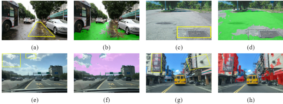
FIGURE 1. Four sources causing invalid object segmentation. (a) Falling-leaves. (b) Invalid road segmentation due to (a). (c) Manhole cover. (d) Invalid road segmentation due to (c). (e) Cirrus clouds. (f) Invalid sky segmentation due to (e). (g) Advertisements. (h) Invalid building segmentation due to (g).
