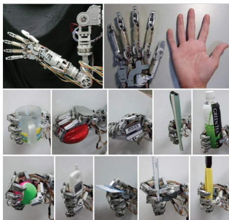
Figure 7. New type of robot arm and its grasping ability
