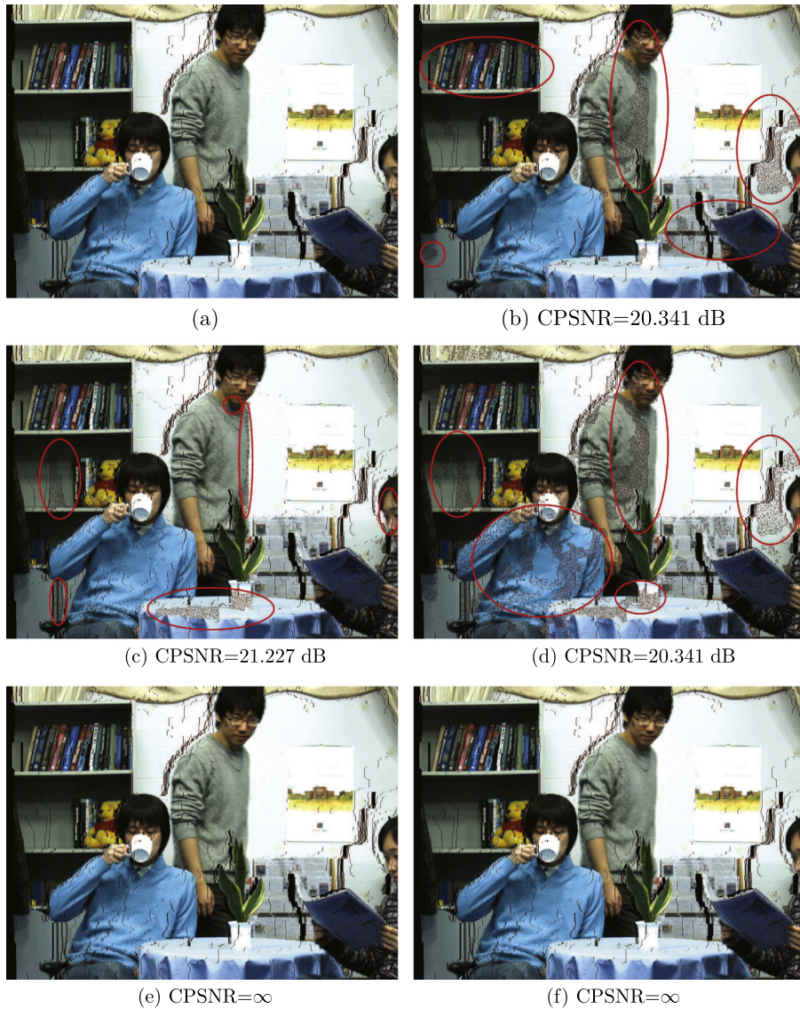
Fig. 7. Rendered virtual views for 3D Newspaper image generated from (a) original depth map and from marked depth maps (with Capacity = 0.9 bpp) by (b) Ni et al.'s method, (c) Thodi and Rodriguez's method, (d) Sachnev et al.'s method, (e) the proposed DNDE-based method, and (f) the proposed DNHM-based method.
