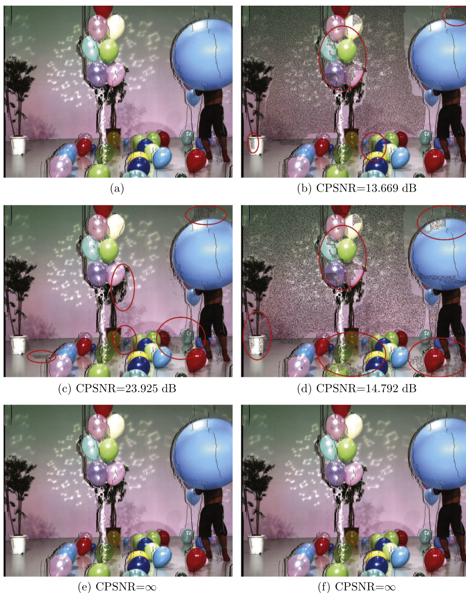
Fig. 8. Rendered virtual views for 3D Balloons image generated from (a) original depth map and from marked depth maps (with Capacity = 0.9 bpp) by (b) Ni et al.'s method, (c) Thodi and Rodriguez's method, (d) Sachnev et al.'s method, (e) the proposed DNDE-based method, and (f) the proposed DNHM-based method.
