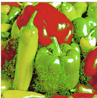
Fig. 8. The over-segmented result after performing the seed-based region growing phase on the enhanced Peppers image in Fig. 6(b).
