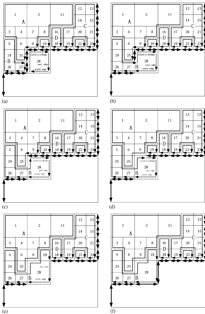
Fig. 7. A simulation of Leaf.Operation for block 28: (a) create block 28; (b) after merging block 28 and active region B; (c) after merging active region A and B; (d) after merging active region A and B; (e) after merging active region B and block 10; (f) update segments on the waveform.
