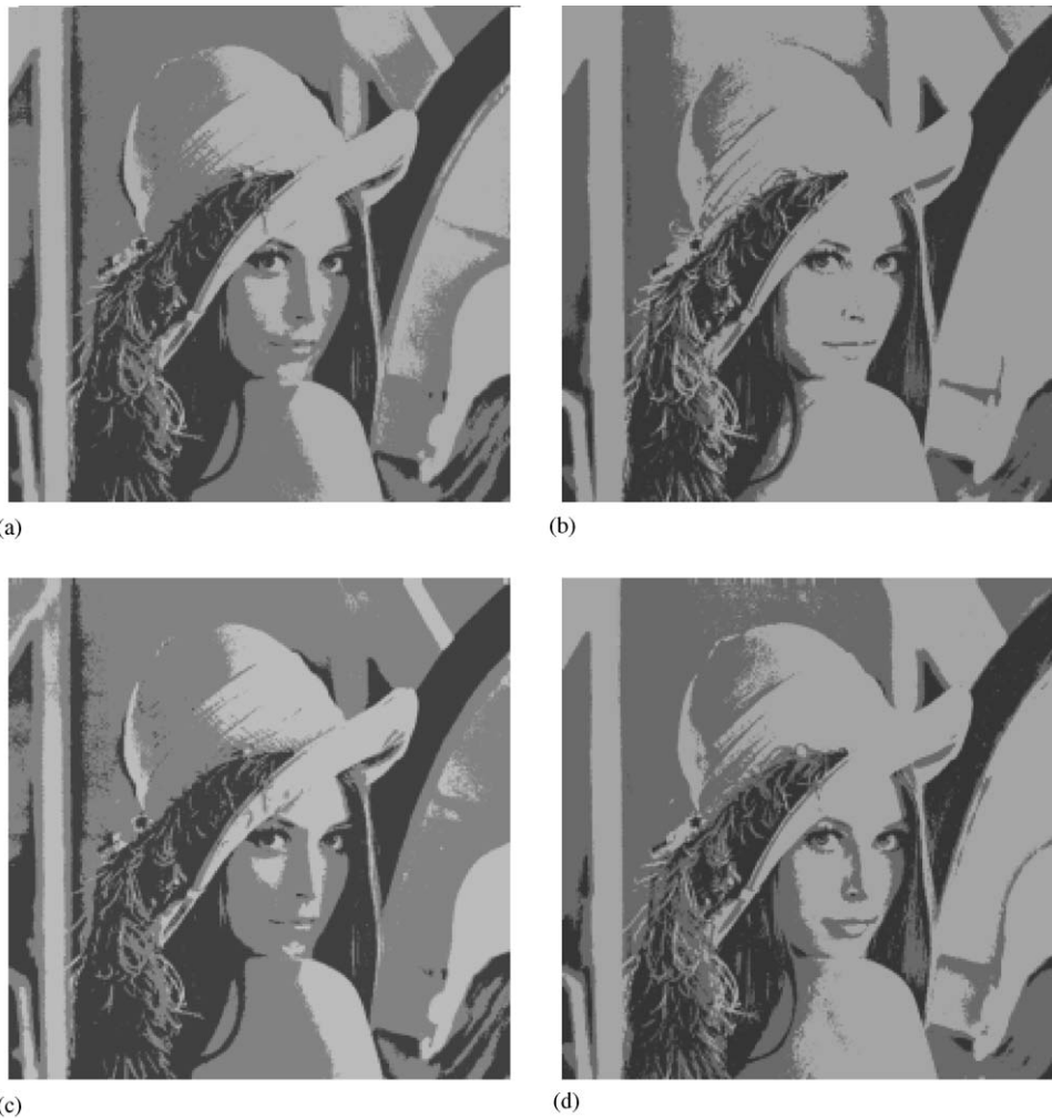
Fig. 7. The thresholded images for Lena with k = 2 ; (a) OT's thresholded image; (b) KI's thresholded image; (c) KA's thresholded image; and (d) OURS1's thresholded image.
